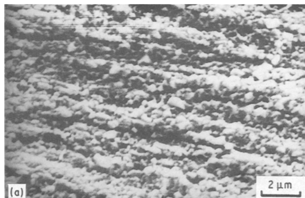
Figure 14 Scanning electron micrographs of (a) selective and (b) nonselective copper-black films (A6).
